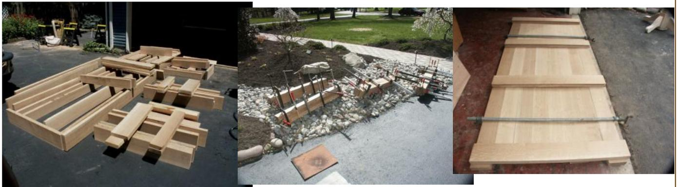
Planks are cut from our predetermined cut-sheets, then blanks are glued up to form the leg structures and pieces requiring lamination of multiple 8/4 layers to reach their final thickness. Everything is proportionate to the table surface, so the surfaces are laid out first in rough form, then the formal joint work begins.
