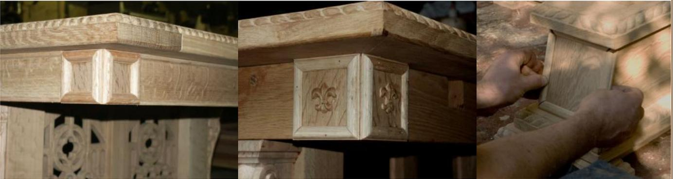
All surfaces that are end grain on exposed faces are covered using an 1/8" thick face plate. Moldings are placed around the corner blocks, feet faces, and aprons, as well as framing the panels. Use of appliques is very common to provide subtle ornate features to the piece.
