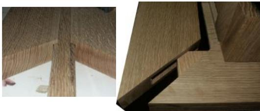
Our tabletops are all tung and groove joints for the panels themselves, as well as a deep 3/4" tung surrounding the panel that is actually a floating joint. In other words, no glue actually holds the main panels of the table, they are free to move about to relieve the tension created by natural expansion and contraction of wood.
