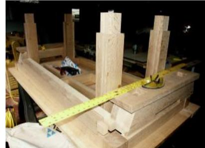
The apron and internal supporting structures (braces) and the top section of the trestle assemblies all reside flat against the tabletop. As these structures take form, the leg spacing and position is naturally established.
